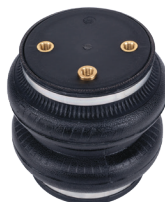
LoadLifter 5000 Zytel® plastic end cap
