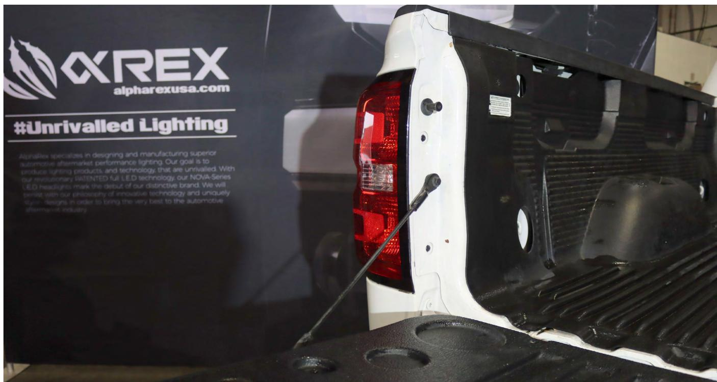
Take out the top and bottom T15 screws from each side of the tail lights.
