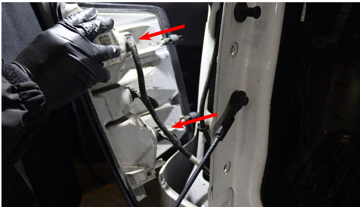
Disconnect the reverse light socket and keep the light bulb for future reinstallation.
