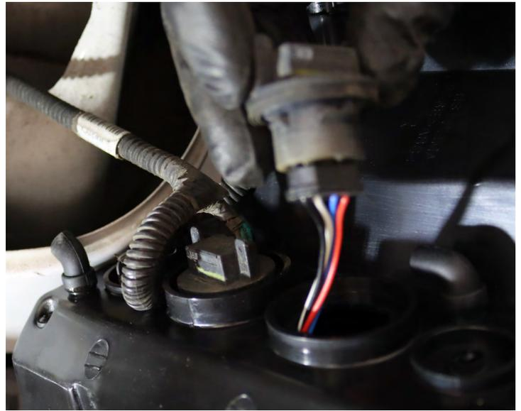
Twist and lock each of the sockets into the new ALPHAREX tail light, ensuring they are tightened and secured. **DO NOT USE DIELECTRIC GREASE!** Follow the same steps for the other tail light.
