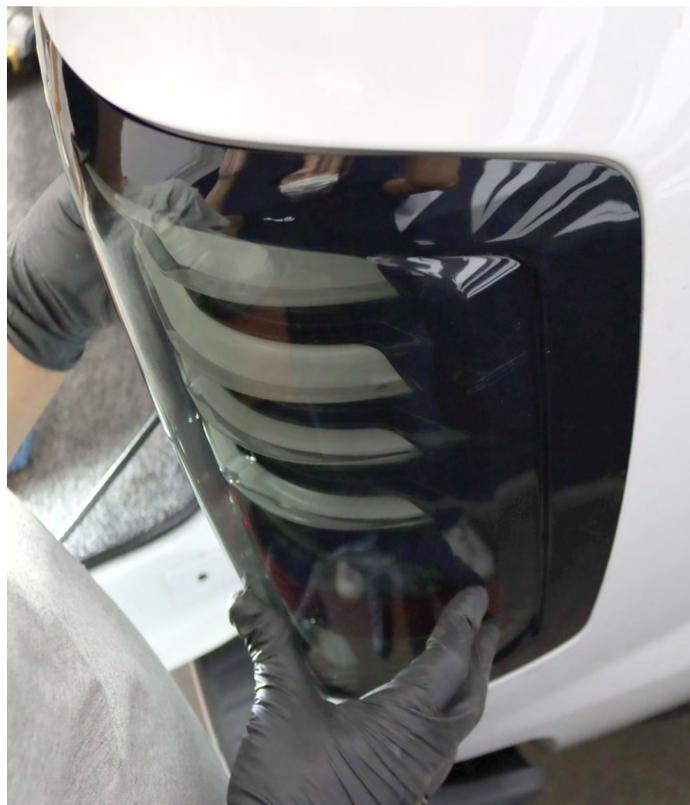
Repeat the same process for the other side of the tail light. NOTE: Whenever using a power wrench, ensure not to overtighten the screws.
