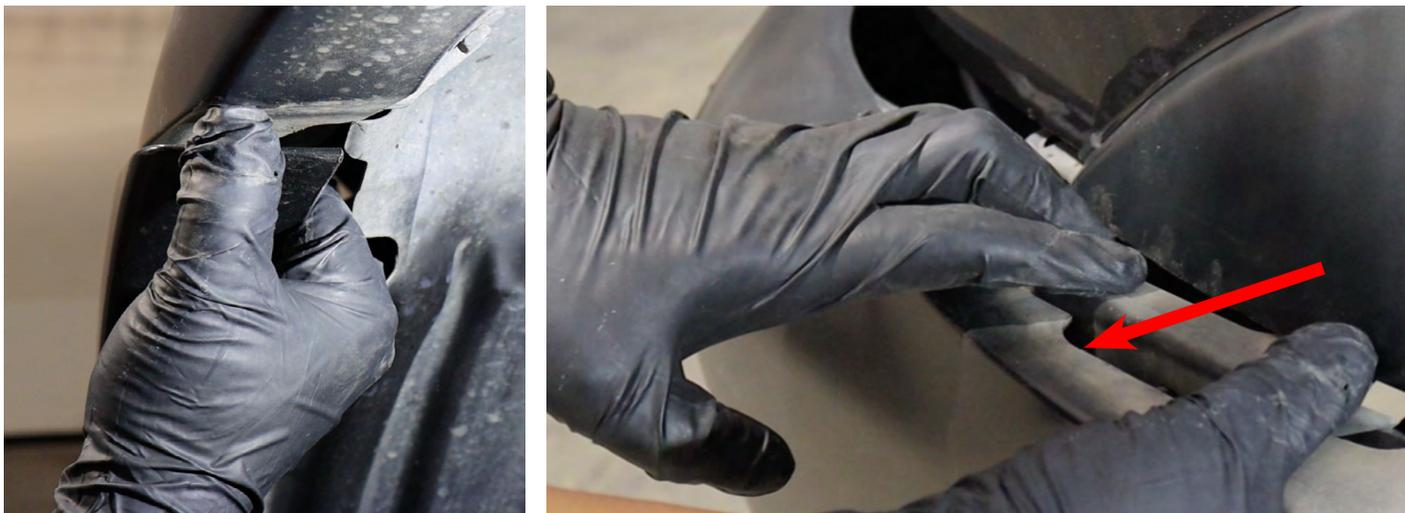
Use a panel popper to remove the two plastic retainers from the front bumper.
