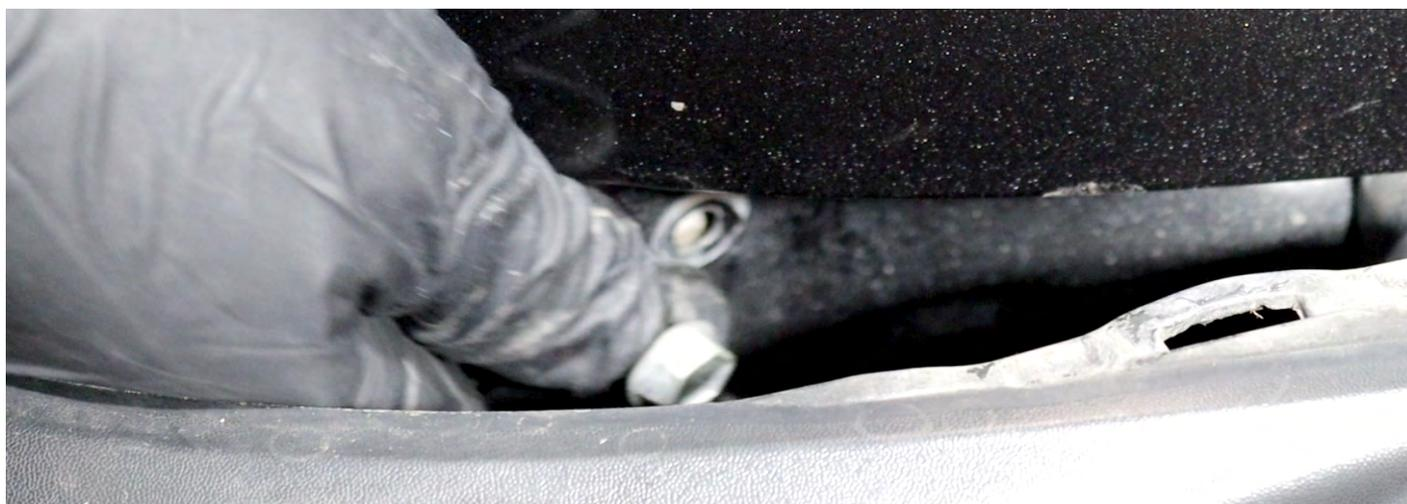
Remove the two 10mm bolts from the top of the headlight.
