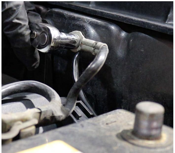
Next, route the fuse tap (grey) wiring through the vehicle's firewall to reach the driver's under-dash fuse box.
