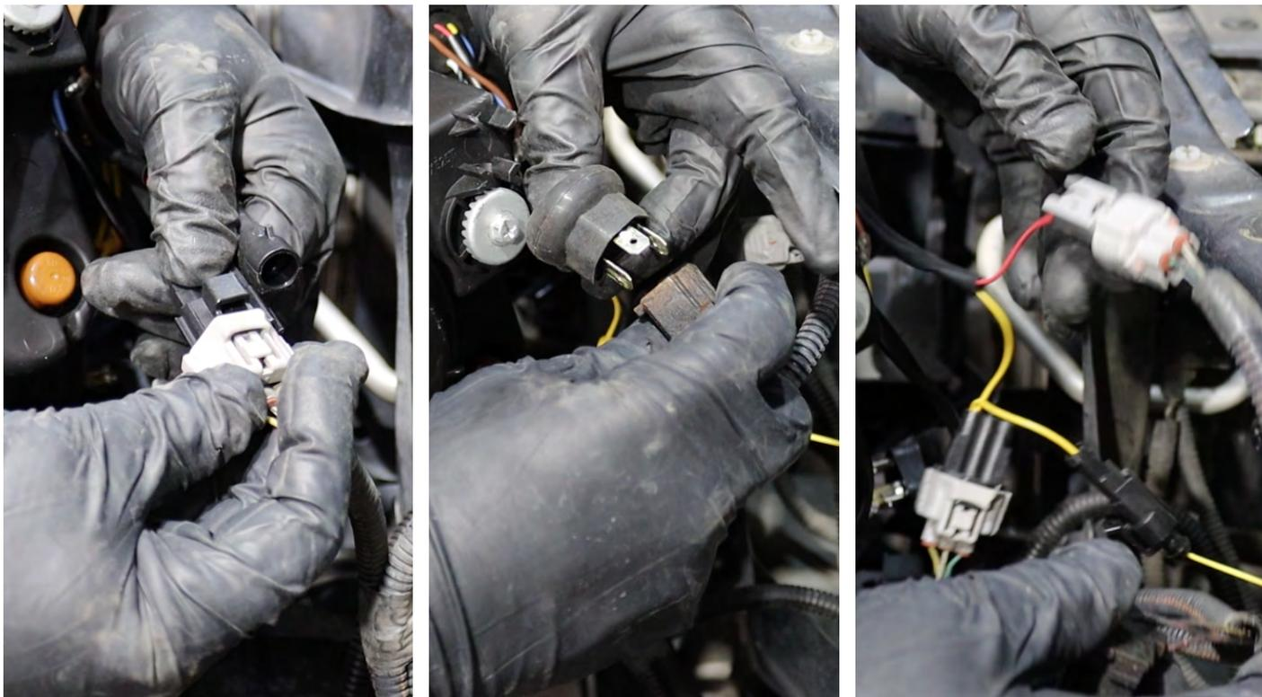
Attach the harness to the daytime running light connection on the back of the headlight. Repeat the same steps for the other side of the headlight.
