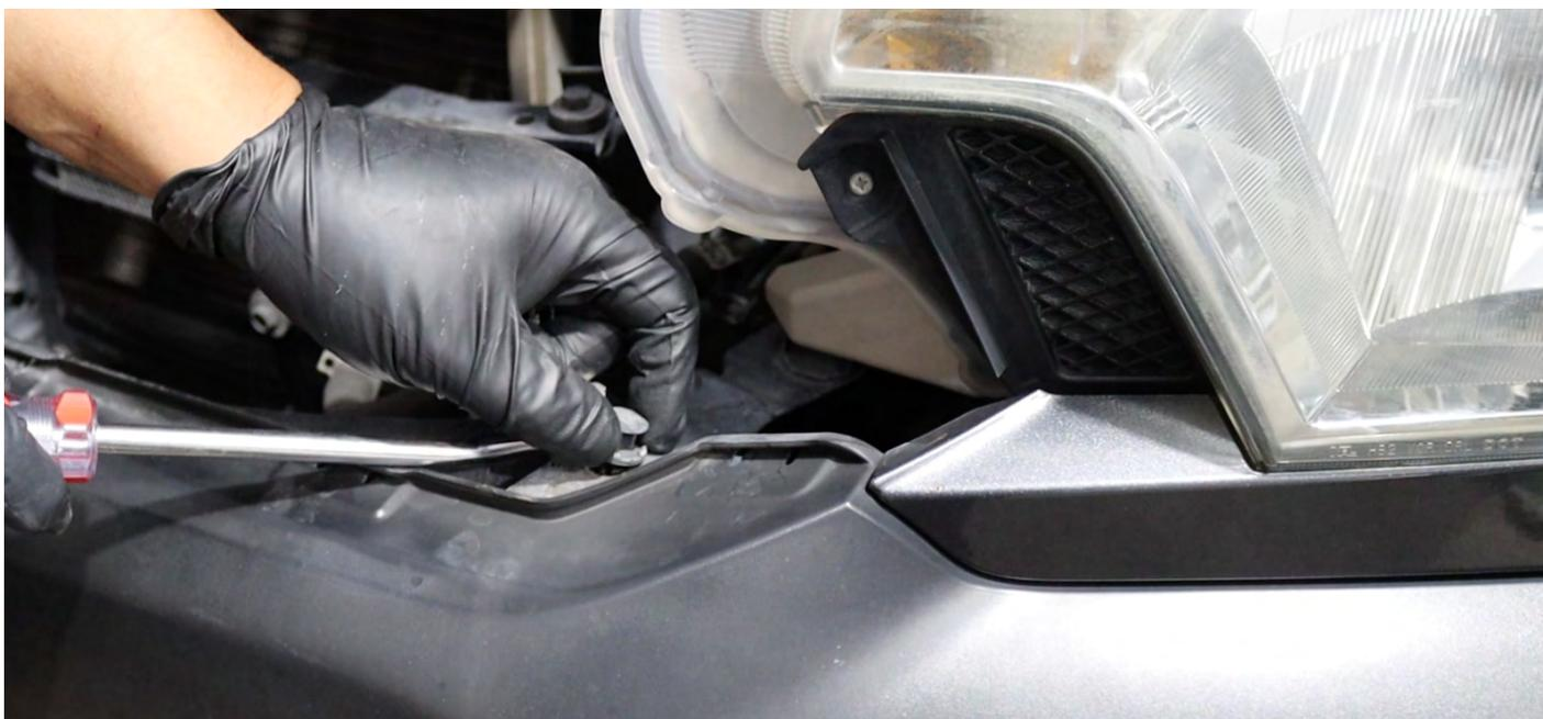
Loosen and release the bumper until you have enough space to reach the bottom of the headlight's bolt. Repeat the same steps for the other side of the bumper.
