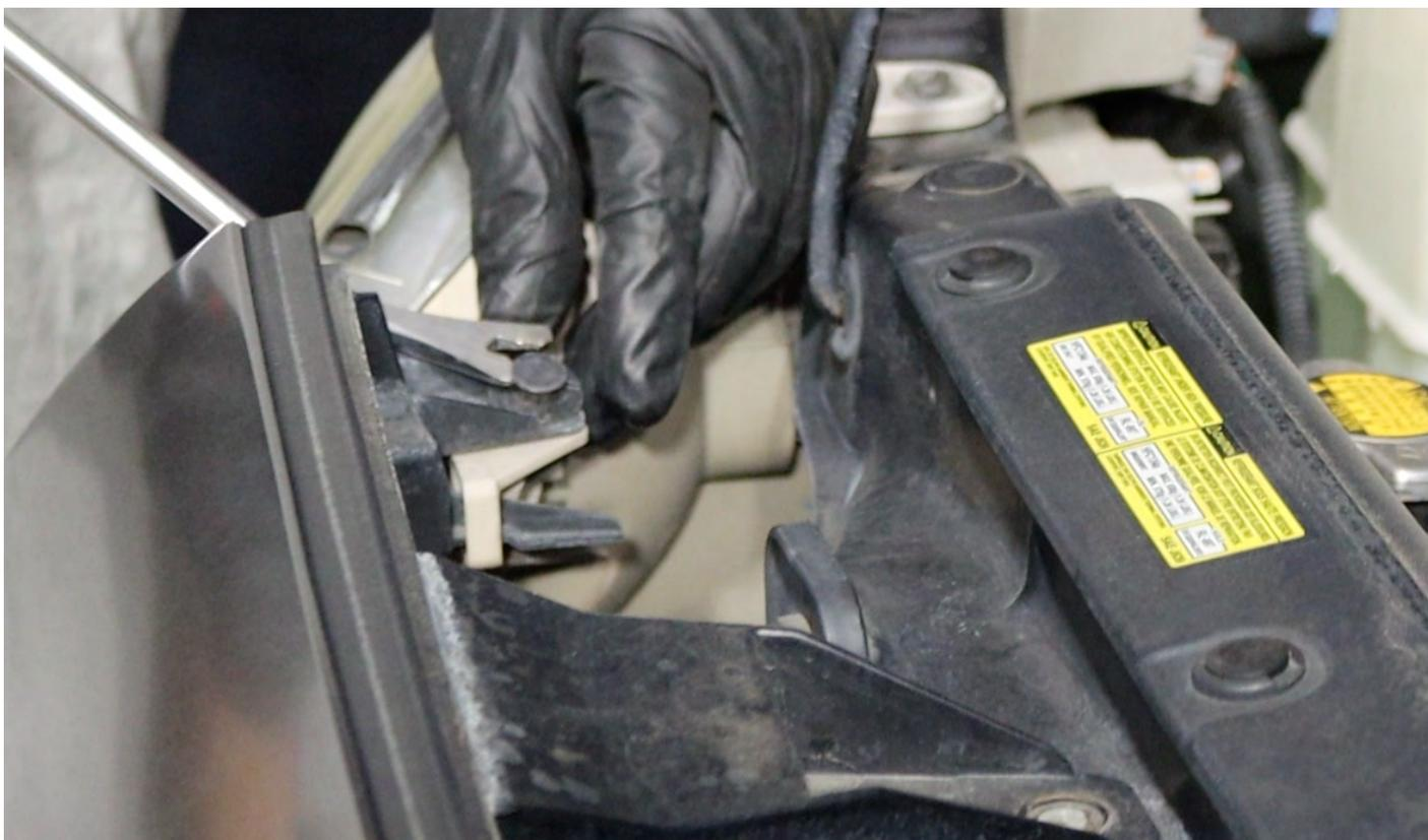
After removing the bolts and plastic retainers, gently pull the grille outward towards you to remove it.
