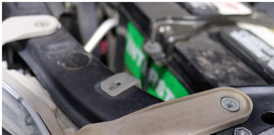
Use a panel popper to lift the headlight and release it from the mounts.
